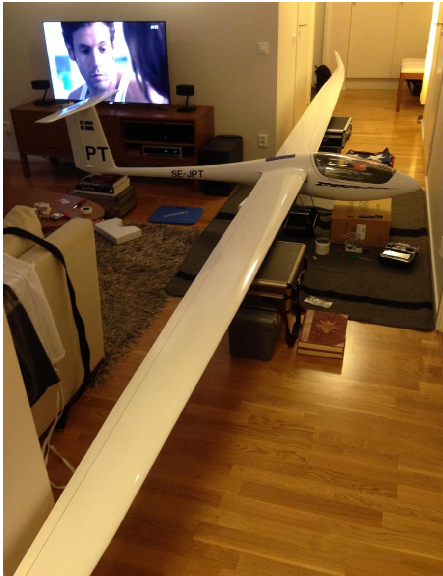
Figure 66. ASH31 on top of CG stand from Great Planes.
