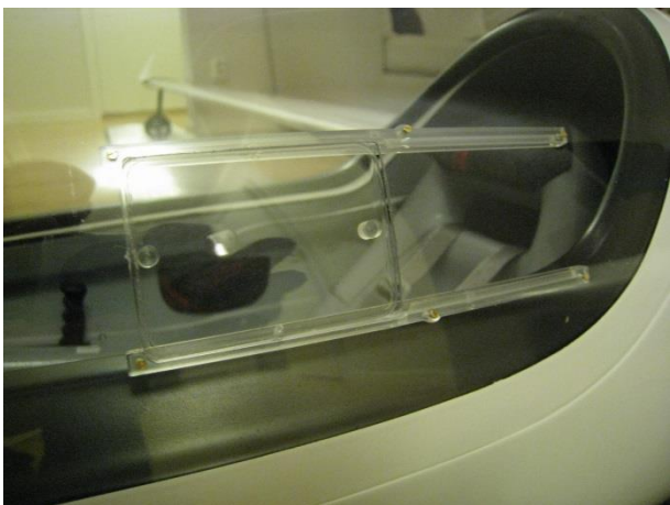
Figure 6. Close up of sliding window.
