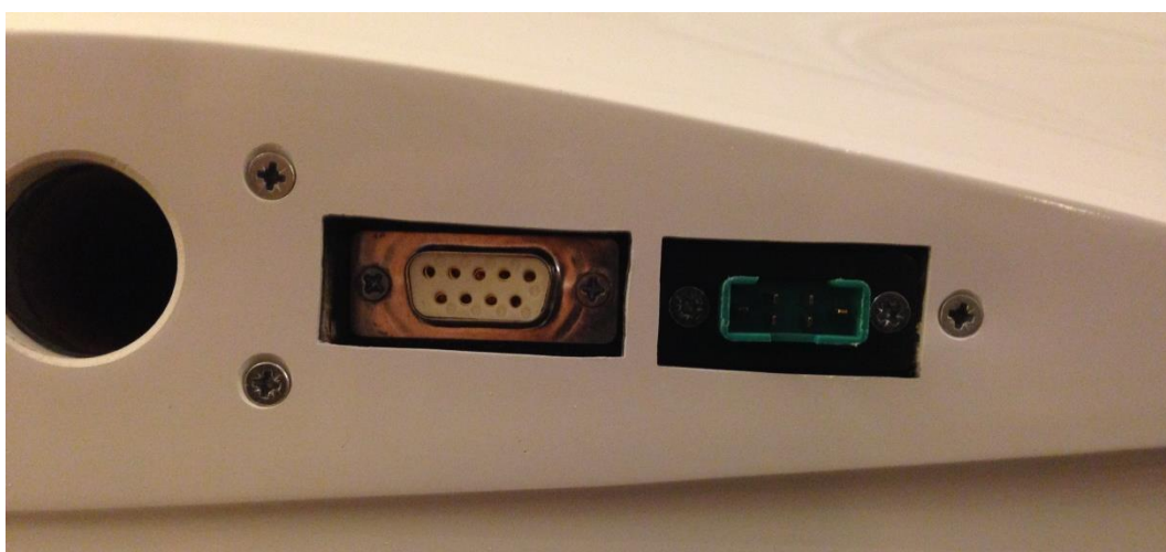
Figure 29. Finished servo-connector support from outside securely fastened using three screws.
