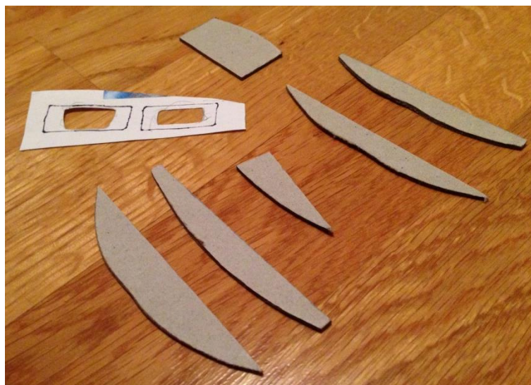
Figure 31. Cardboard templates for servo connectors, tow release servo, battery tray, rudder servo and PowerBox.
