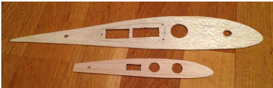
Figure 23. Inner and outer wing profile templates for servo connectors.
