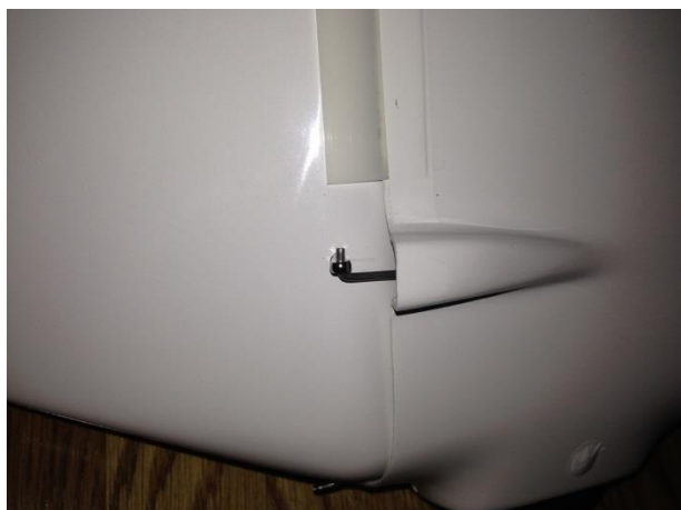
Figure 17. Rudder with linkage.
