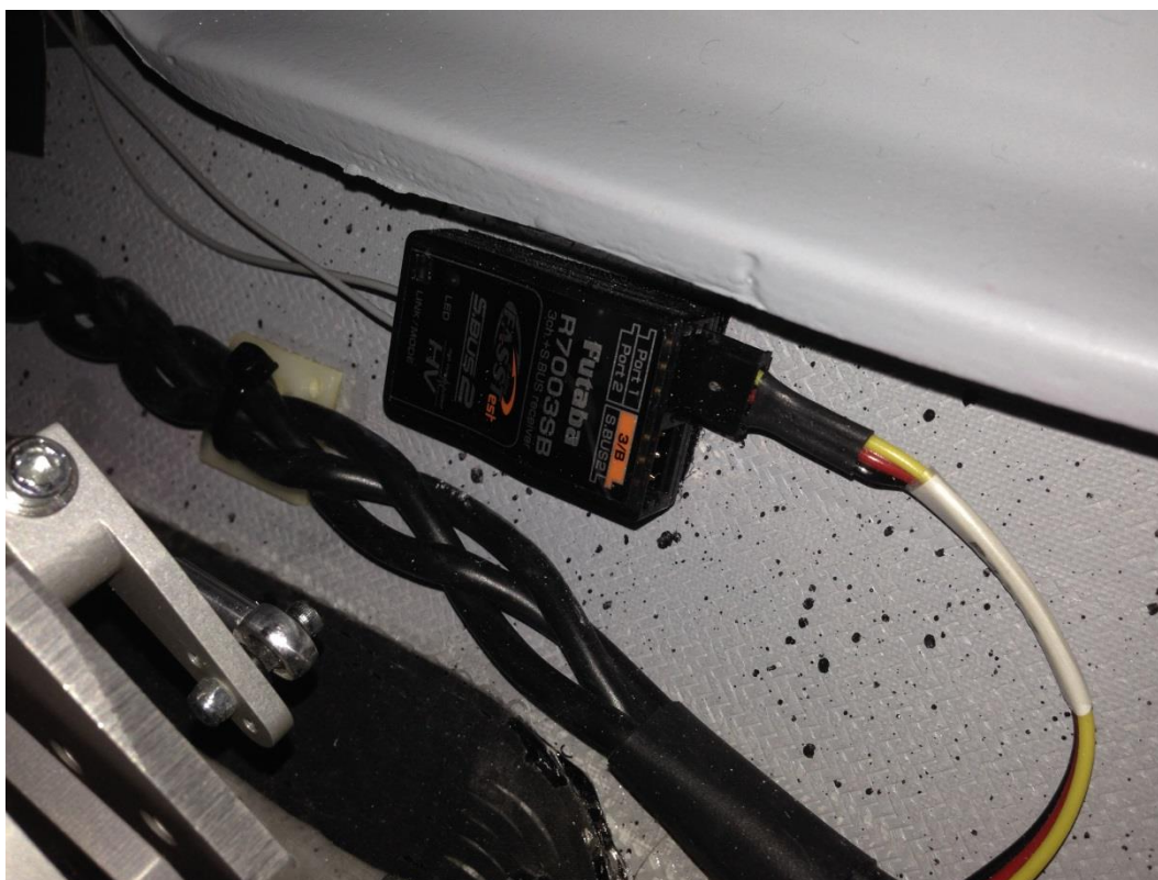
Figure 50. Secondary receiver location next to the landing gear on the left side of the fuselage.
