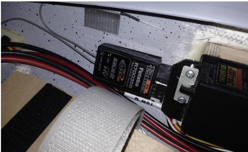
Figure 49. Primary receiver location with telemetry input from the Powerbox and the voltage sensor.
