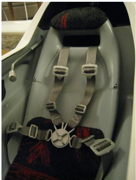
Figure 9. Seat with harness.
