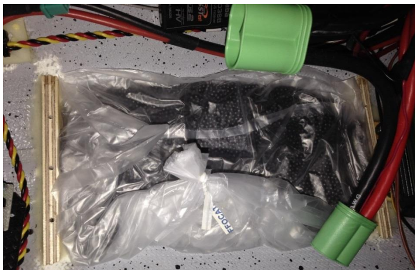
Figure 69. The lead shots (568 g) fit perfectly below the motor battery tray.
