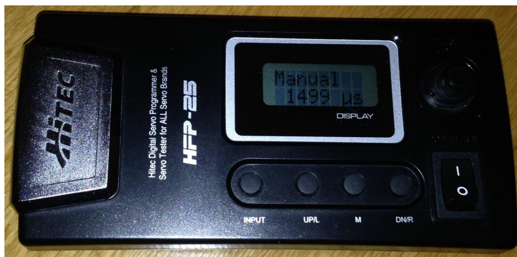
Figure 35. The HFP-25 from Hitec is a valuable tool for easy servo installation.
