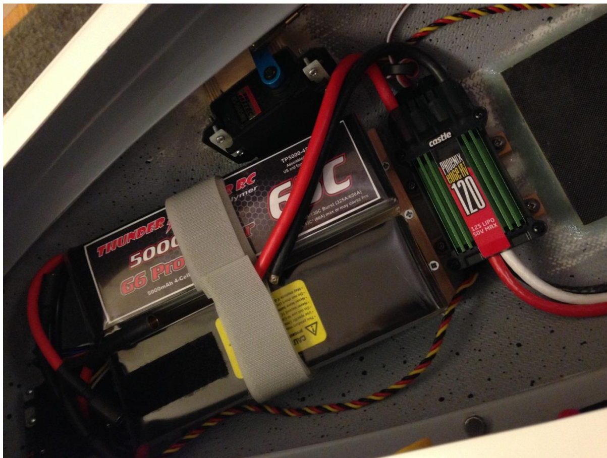
Figure 34. Motor batteries test fitted on top of battery tray, rudder servo (HS-5645MG) in servo frame from Paritech and the Castle Creations Phoenix Edge HV 120 mounted to its support ribs.
