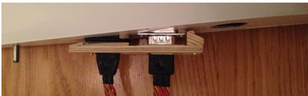
Figure 26. Internal servo-connector support from plywood with standoffs.
