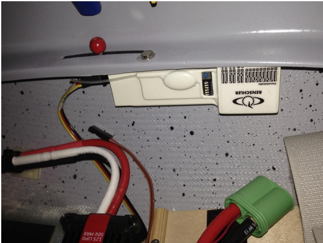
Figure 51. Mounting location of the Picolario system.
