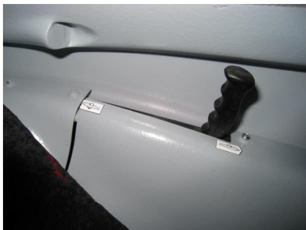
Figure 11. Retract mechanism lever.
