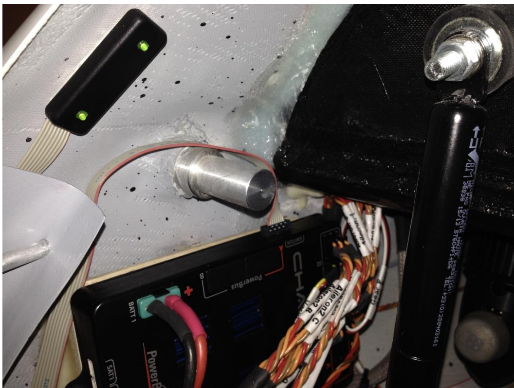
Figure 46. Powerbox Champion SRS and magnetic On/Off switch.
