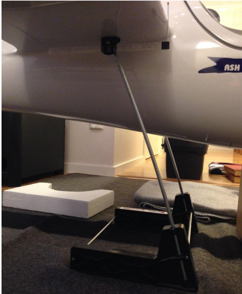
Figure 67. Recommended CG is located 90 mm from leading edge.
