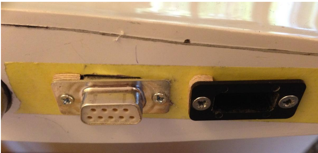
Figure 20. Front view of 9-pin d-sub and short connector frames for multiplex connectors.
