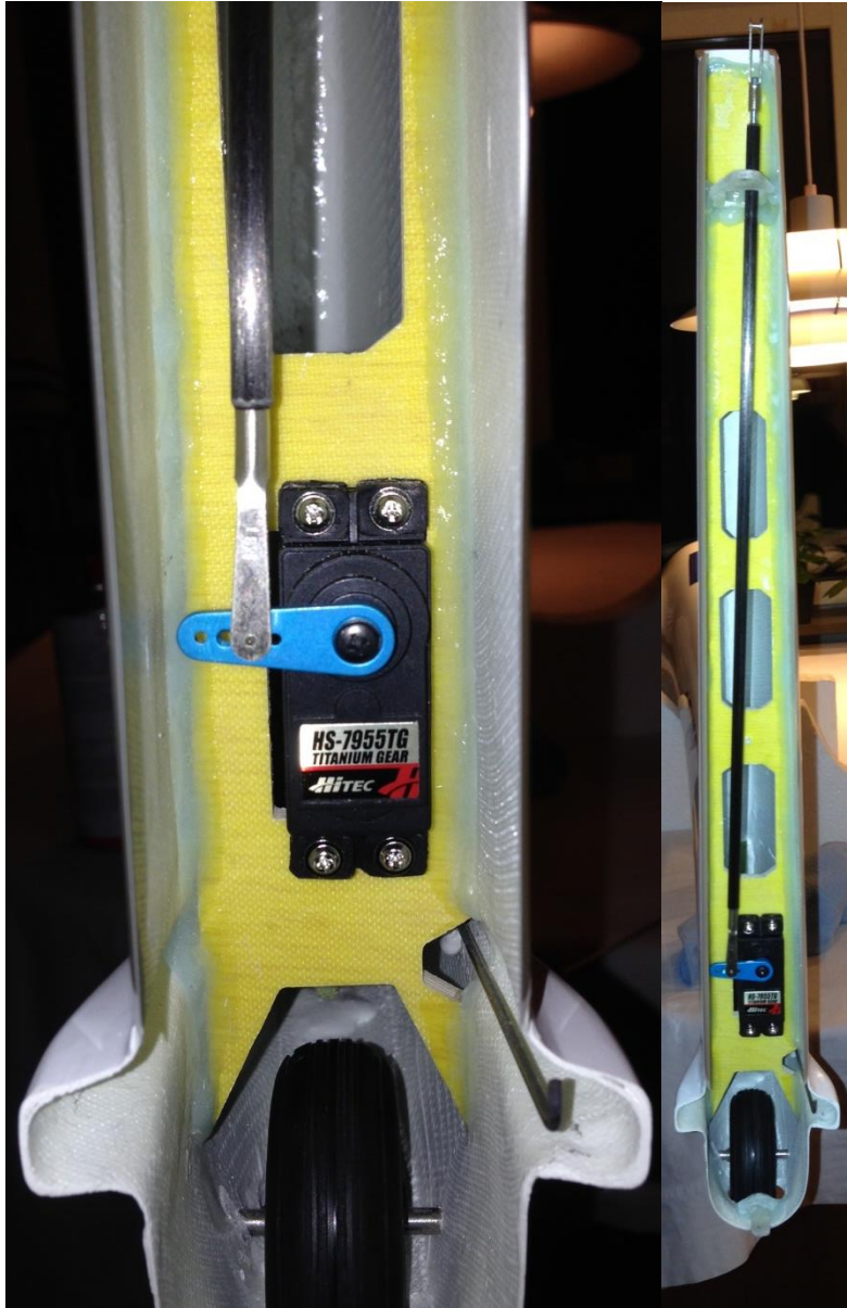
Figure 44. Elevator servo and pushrod installation.
