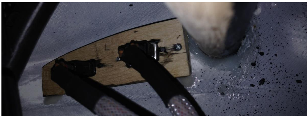
Figure 27. Servo-connector support from inside fuselage.
