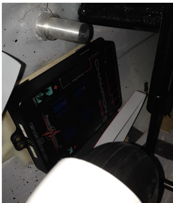
Figure 33. PowerBox Champion SRS mounted on the support.
