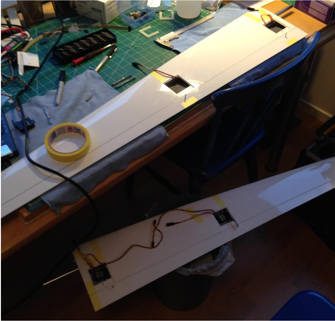
Figure 42. Outer wing panels with HS-5125MG servos. The servos are synchronized using the PowerBox Champion.
