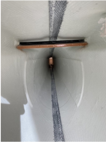
Carbon tube and hard wood piece at the rear of the wing.
