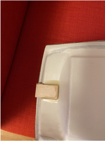
Plywood piece glued to the front of the canopy.
