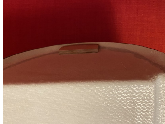
Plywood piece glued to the back of the canopy.
