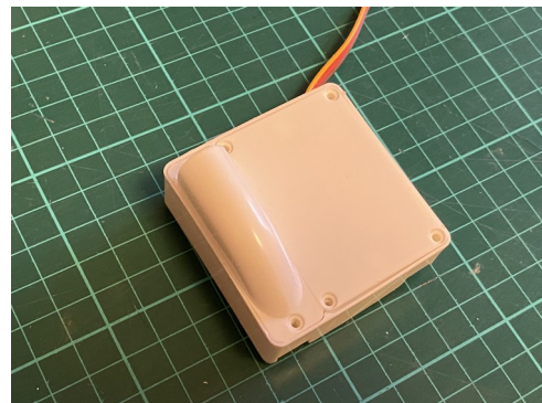
A flap servo seen from the top.
